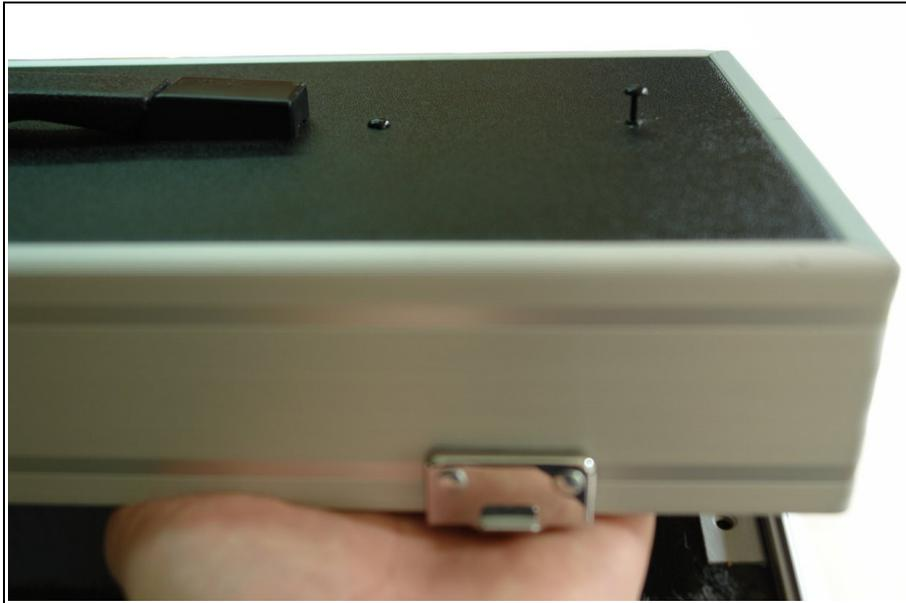
Picture 6. Fixing the analogue outputs module by means of the mounting pins.
